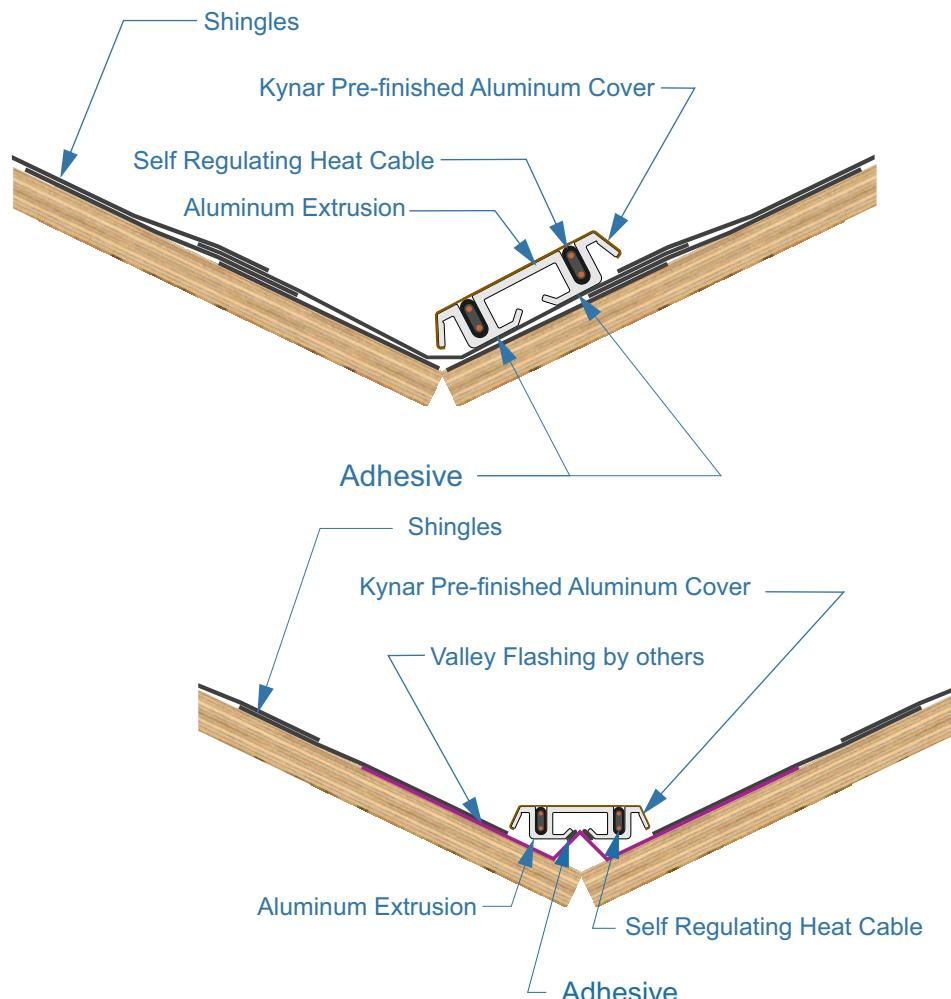
**NOTE:** Some roof assembly features omitted for clarity. IceBlaster products are fully compatible with most roof styles and systems. IceBlaster Valley Panel can be installed metal W valley styles or shingle woven valley styles.
