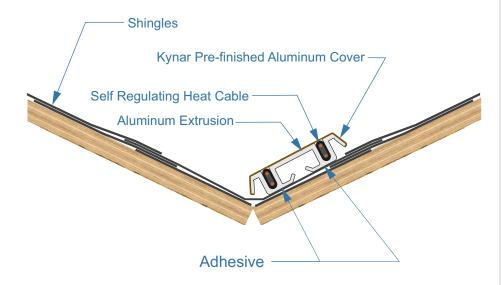
**NOTE:** Some roof assembly features omitted for clarity. IceBlaster products are fully compatible with most roof styles and systems. IceBlaster Valley Panel can also be installed metal W valley styles.
