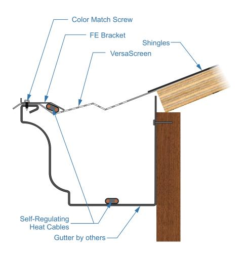
**NOTE:** Some roof assembly features omitted for clarity. VersaScreen Pro is designed to fit a variety of gutter style and installation methods. VersaScreen and IceBlaster products are fully compatible with most roof styles and systems.
