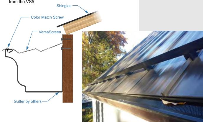
**NOTE:** Some roof assembly features omitted for clarity. VS5 is designed to fit a variety of gutter style and installation methods.
