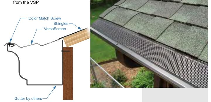
**NOTE:** Some roof assembly features omitted for clarity. VSP is designed to fit a variety of gutter style and installation methods. VSP is perfect for gutter installations where a gutter apron is used and the screen can be slid under the first course of shingles.
